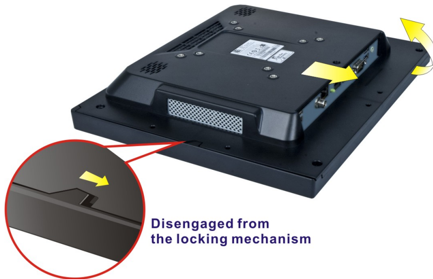
Figure 3-4: Remove the Back Cover
