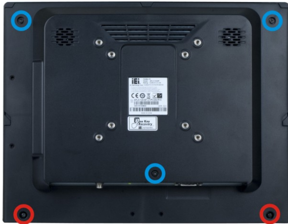
Figure 3-2: AFL3-12A-BT Back Cover Retention Screws
