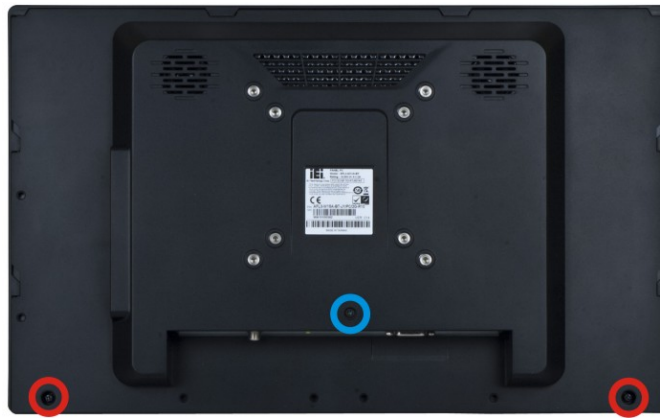
Figure 3-3: AFL3-W15A-BT Back Cover Retention Screws
