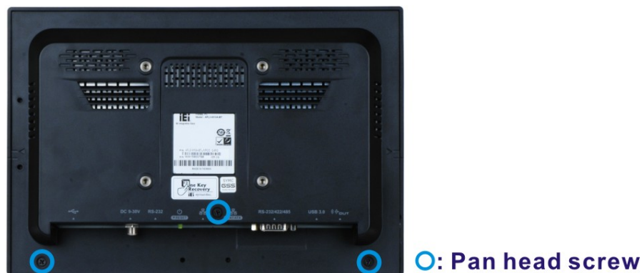
Figure 3-1: AFL3-W10A-BT Back Cover Retention Screws
