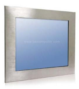
The PMS7715 is a Touch Panel PC comprised of an Intel 3rd Generation Core i5/i3 or Pentium processor and two 240-pin DDR3 DIMM slots for up to 16GB maximum system memory. The front stainless steel front bezel is IP65 rated and houses a 15" LED backlight 400nit LCD with a resolution of 1024 x 768. The touch screen is an ELO 5W Analog resistive type using USB interface. The dimensions of this Panel PC are 402.8 x 303 x 85.8 mm and weighs in at 7.5 kg.
