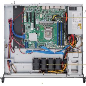
ATX (12" x 9.6") or uATX (9.6" x 9.6") Board Form Factor
